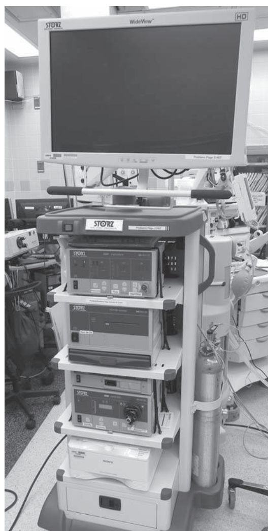
Figure 81.1 Modern video tower fitted with monitor, light source, image processor, and recording device.
